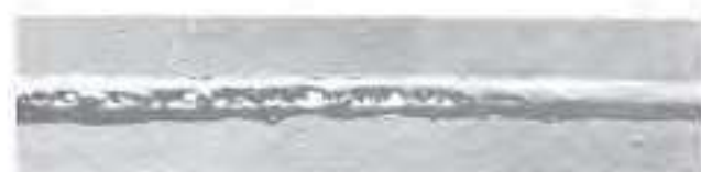
FIGURE 6 — Dirty flux can cause severe porosity.
