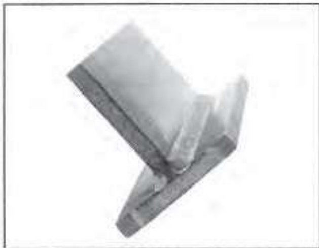
\frac{1}{2} " (12 mm) flat fillet welded at 540 amps at 15 in./min (0.38 m/min) with 3- \frac{1}{4} " (82 mm) stickout using a hand-held gun.
