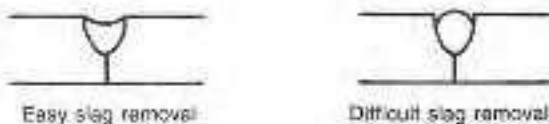
Figure 7 — The first pass of a two pass weld should wash up to the edges for best slag removal.
